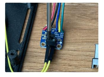
The wires are a bit of a tight fit, so it's easier to install them in the MAX98357 terminal first. Place the wires in the appropriate terminal so that they have enough length once installed.
