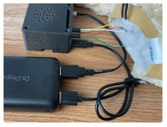
Connect the USB cable between one port of the power Bank and the Raspberry Pi.
