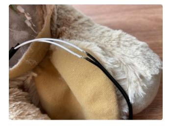
Strip, tin, and solder the harness to the foot button wires. The specific wire doesn't matter since pushing the button connects them together.
