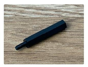
Continue tightening about an additional 1/6 turn until and line up the flat edges. Don't over-tighten or the plastic could break off. The idea is to have more friction between these two standoffs than you will have with the standoff you are installing.
