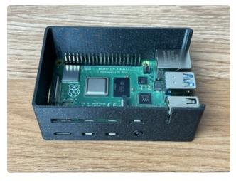
Insert the Raspberry Pi 4 in the bottom case. Make sure you don't have a MicroSD card inserted! You'll want to have the A/V ports go in first before pushing the other side down so that it is sitting flat.
