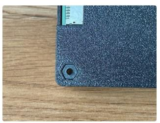
Place a nut into the hex insert on the bottom of the case.
