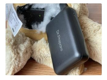
Place the enclosure into the bear next. There's a small hole so you can see the status lights. Having that face down lets you easily know if the Pi is powered up or not. Continue adding stuffing, but leave room for the battery.
