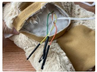
Strip and tin the wires inside the bear. Very carefully solder the wire extensions to the motor wires sticking out. You may want to temporarily remove some of the stuffing to give you more room to work and place some aluminum foil around the area you are working.
