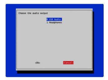
Select System Options→Audio. Make sure USB Audio is selected and then tab over to Ok to select it. After that, you can exit to the command line and that's it.
