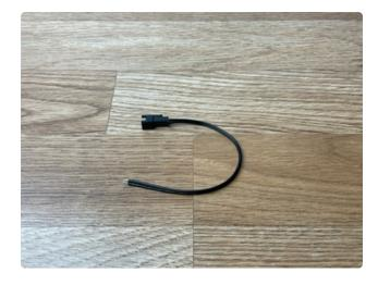
Prepare the receptacle half of the connection by stripping and tinning the wires.
