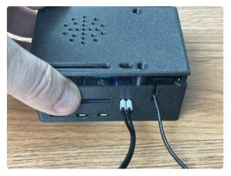
Install the lid by placing it directly over the case bottom and lowering it. If the strain relief knot is in the way, you can push it in temporarily while placing the lid. It may take a little bit of adjusting if some of the wires are in the way.
