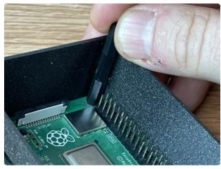
Screw the standoff into a nut. When it is tight enough, just hold it in place with a finger or flathead screwdriver and unscrew the tool from the installed standoff.
