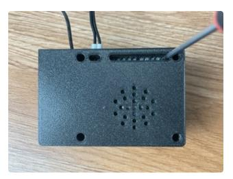
You may also want to loosen the appropriate screws for the motor wire terminals. However, those can be installed after the case is assembled.
