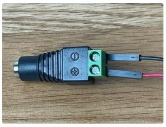
Install the jumper wires in the female DC power adapter. It's a good idea to use different colors so it's easier to tell which side is positive and which side is negative.
