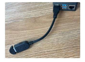
If you would like to be able to control where the sound is picked up, you could use a simple USB extension cable.
