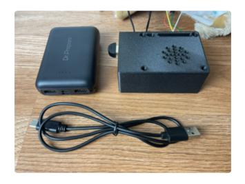
To power the Raspberry Pi and motors, you'll want the USB power bank along with a short USB cable. If you don't have any extras, you can use the USB cable that came with the power bank.
