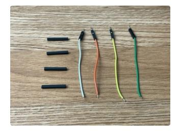
You'll want to cut, strip, and tin 4 wires to match the motor wires. You will also want to cut 4 pieces of heat shrink tubing. Place the heat shrink on the wires now so you don't forget later.
