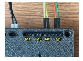
When you connect the wires from the bear, the wire order is important. Install the wires to the M2 and M2 terminals as shown in the photo.
