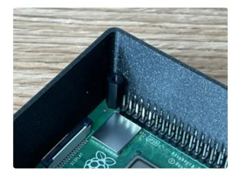
Install a standoff through the Pi and into the nut you inserted using a tool.
