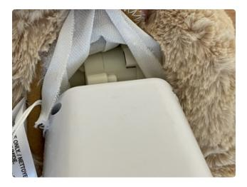
The housing is attached further up with a bunch of hot glue. Applying some isopropyl alcohol (or IPA) to the glue with a cotton swab or something similar will cause the glue to become brittle and less adhesive. The higher the concentration of IPA, the better it works. Don't forget to remove the glue on the lower white wires.
