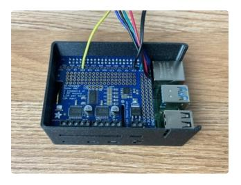
Place the motor HAT onto the Pi. You can use the upper left side of the case (the corner furthest away from any ports) to easily align the GPIO headers.
