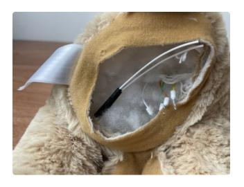
Place some heat shrink tubing on the foot button wires. Since the wires are already separated, it make things a lot easier.
