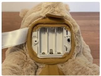
The fabric around the electronics housing should now be free to pull away. Go ahead and pull the housing out of the bear.
