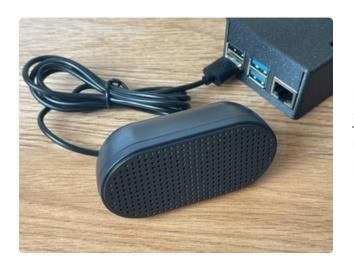
If you went with the easier install option, just plug the speaker into one of the USB ports of the Raspberry Pi. We'll show you how to configure it later.
