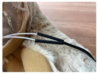
Slide the heat shrink tubing over the soldered wires and heat it up. Since the wiring isn't as short as the motor wires, this is much easier.
