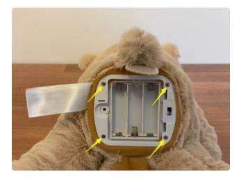
Remove the 4 screws and set them aside. Then remove the cover. You may need to pry it a bit.
