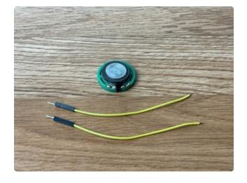
Prepare two more wires and desolder the ones that come with the speaker.
