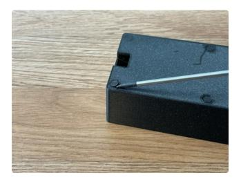
Make sure to remove any supports. A small flathead screwdriver or so small needle-nosed pliers should work well.
