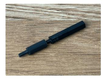
To use, just thread the standoff that you are installing onto the threads of the tool you assembled. Just use a minimal amount of friction since you want it to come off of the tool when it's installed.
