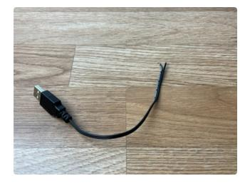
Cut the cable with about 6 inches of wire length from the USB plug and strip the ends.
