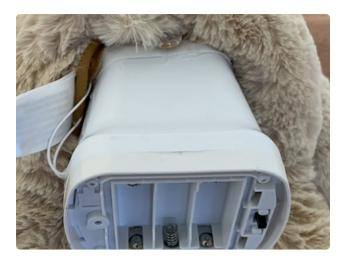
To expose the housing, first carefully push the cloth around the housing up so that the bottom half inch of the housing is exposed. Then push it up the rest of the way.
