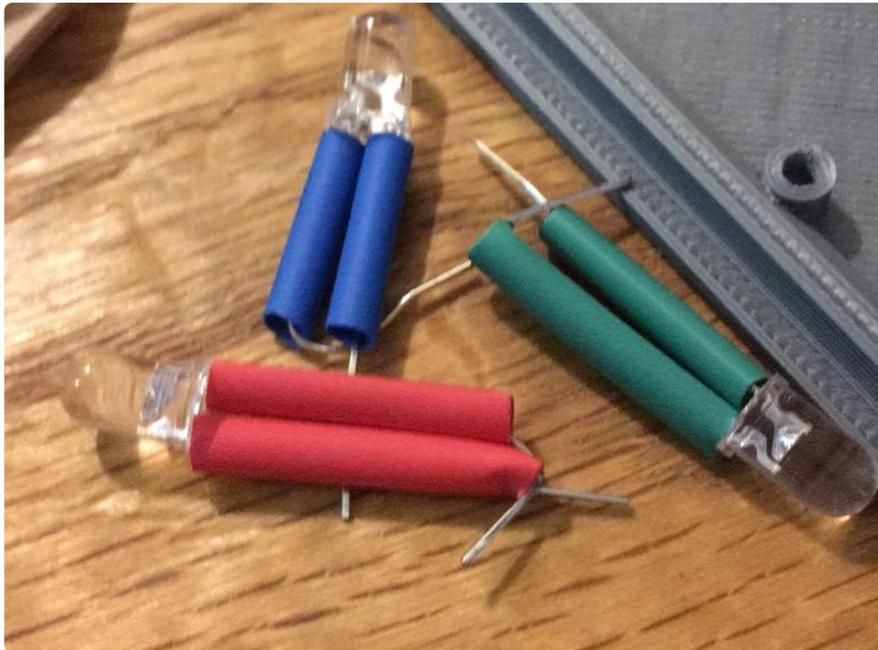
When laying out wire and soldering, make sure you use long enough lengths of wire for the potentiometers, NeoPixel strip and individual LEDs so that when you insert them into the case they have enough room and none of their connections are being stressed.
