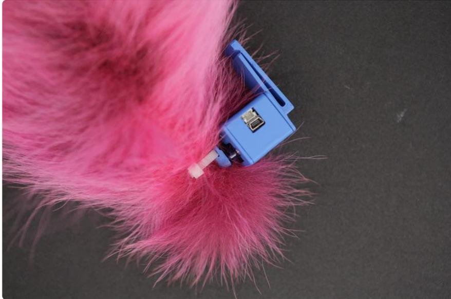
When you run the software presented on the next page, you might find the tail is off-balance. Easily fixed! Just wait for the tail to come to rest, disconnect power, then unscrew the servo horn (the little piece to which our tail is tied) and reinstall it in a neutral (centered) position.
