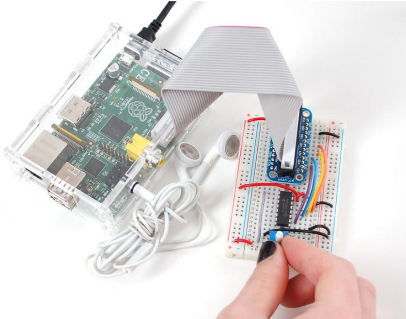
Teaching the Raspberry Pi how to read analog inputs is easier than you think! The Pi does not include a hardware [analog-to-digital converter](https://adafru.it/eYp) (<https://adafru.it/eYp>), but an external ADC (such as the [MCP3008](http://adafru.it/856) (<http://adafru.it/856>)) can be used, along with some SPI code in Python to read external analog devices.
