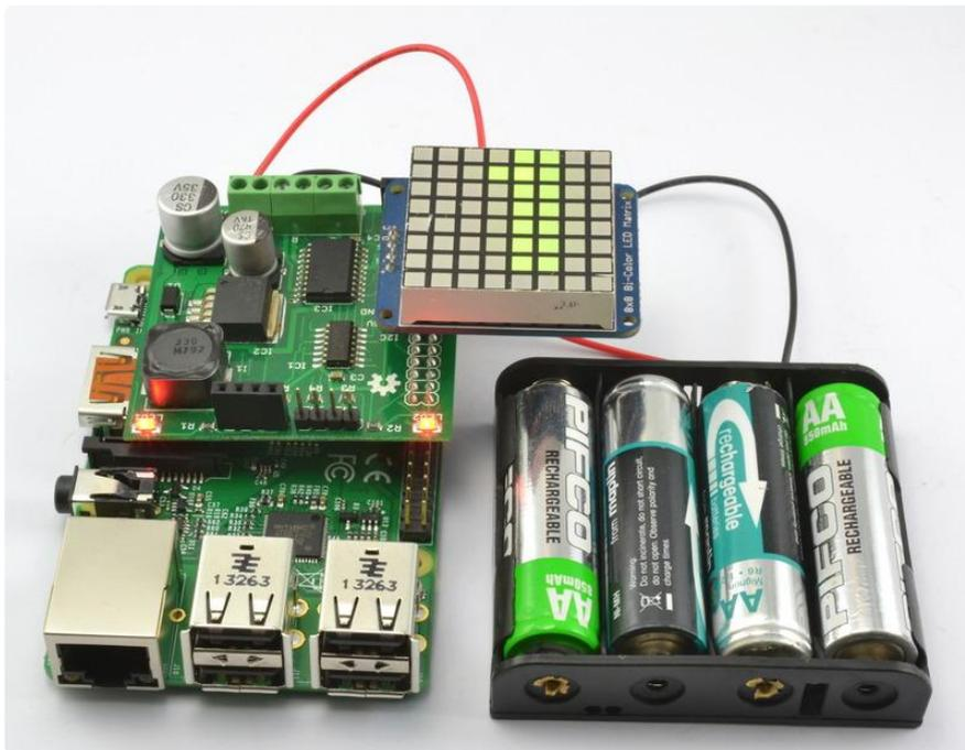
In this tutorial you will learn how to use the RasPiRobot Shield and an AA battery pack to make a portable Raspberry Pi powered display. The display will show the current time as scrolling text, but the project can easily be modified to display other scrolling text messages. The parts used in this project are listed in the Featured Products bar on the right of your screen.
