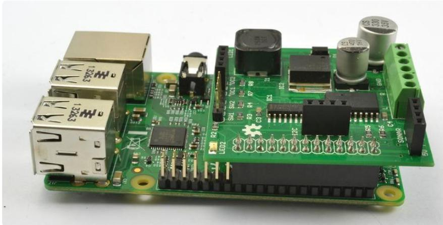
If you are using a Raspberry Pi model B, then the RasPiRobot Board V2 will fit over all the GPIO pins, as shown below.
