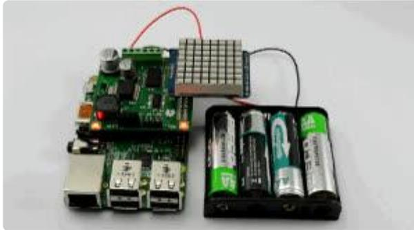
Although the RasPiRobot Board is primarily intended as a motor controller, it also includes a high current switch mode voltage regulator that allows you to power a Raspberry Pi from a wide range of battery types.
