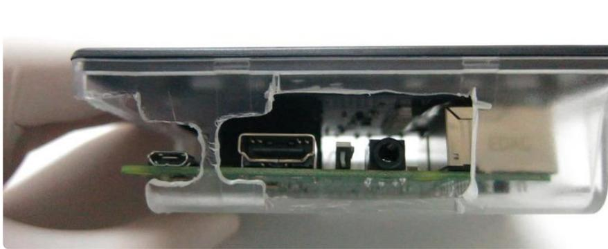
Once cut, attach the PiTFT to the facade of the case using the included screws and button covers. You'll need to remove the PiTFT from the GPIO pins of the B+ to accomplish this, and then reattach the B+ to the now installed display.
