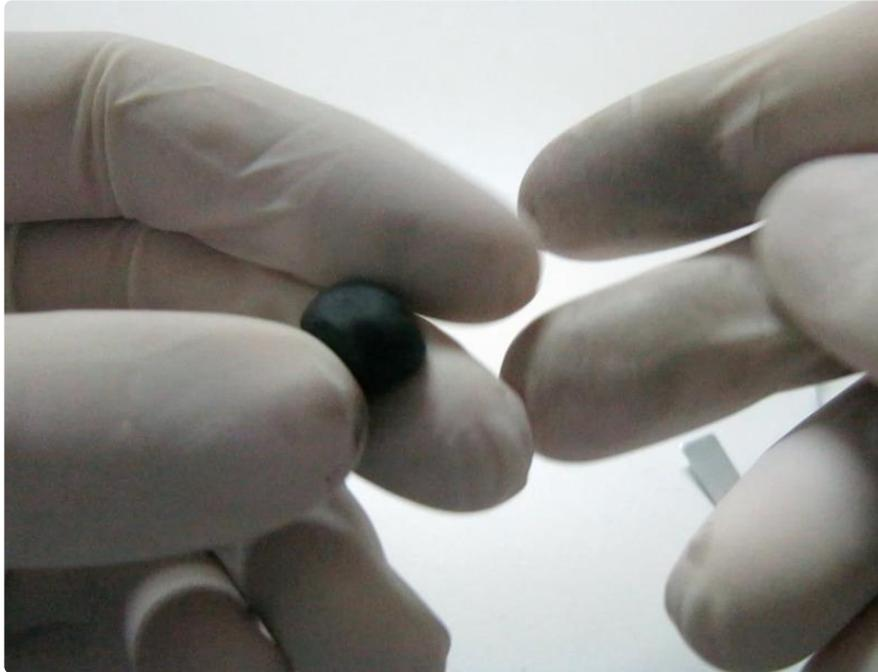
Tear off small portions, roll it into a ball until it's activated, and then into a small tube. I recommend trying to keep everything smooth from the beginning, so that it doesn't leave tiny splotches or jagged lines.
