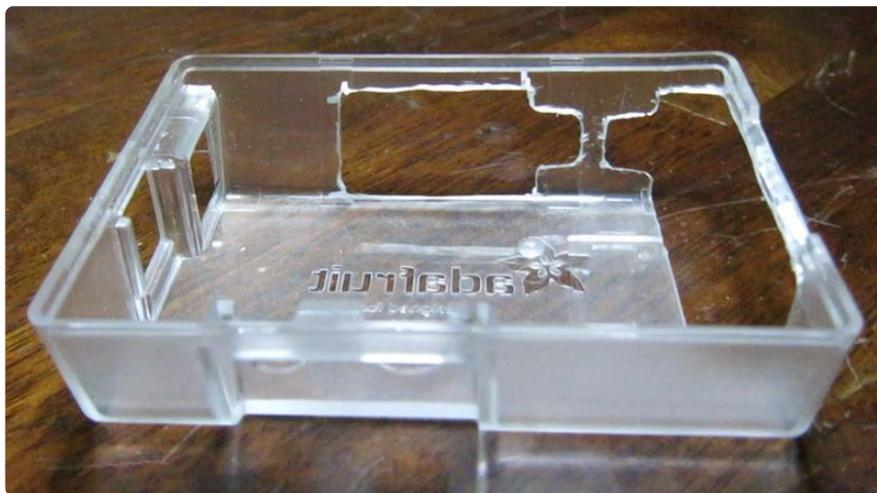
Special consideration is required for the space around the USB jack and HDMI jack. The sideways-H shape outlined in the photo, separating the two cut-outs, is to keep the structural integrity of the case as high as possible. By leaving a small bridge, the case doesn't fall in on itself.
