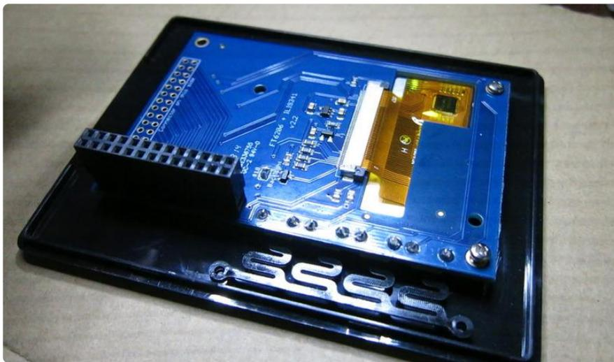
Check your alignment. Plug in the USB and HDMI cables to ensure clearance, and then leave a little extra room for the Sugru finishing step.
