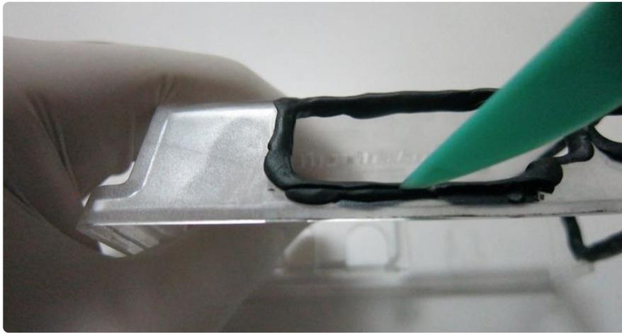
I found the best method was to put a little bit on all the spots to make sure I kept it as thin as possible, and then work my way back around to keep it consistent. You want to finish this entire application within about a halfhour, so the Sugru stays pliable. Don't get up to take a break until you're finished.
