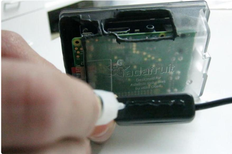
Then, while the case is upright (being careful not to glue your project to the table), place and hold the switch against the base of the case for 45 seconds, to a minute. The glue will have a primary bond, and will be stable enough to allow it to dry.
