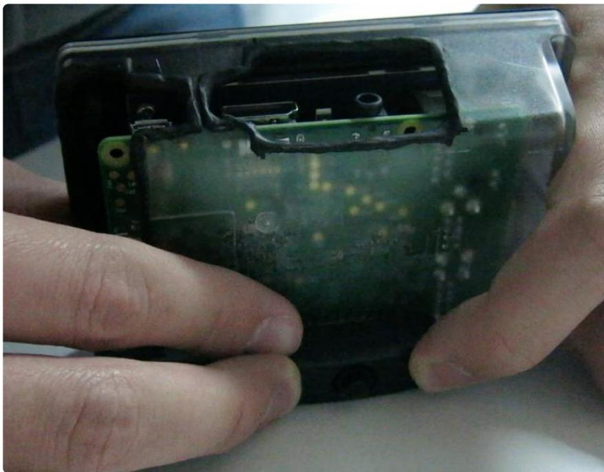
Make sure your orientation is correct on the switch, so that you don't accidentally glue it with the micro-USB end pointing away from the USB port on the RasPi.
