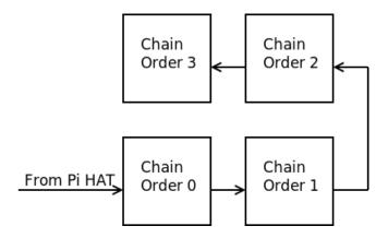
The output of the Raspberry Pi is connected to the bottom left panel, then snakes around through all the panels and ends in the top left. The very first panel connected to the Pi is order/position 0 in the chain, the next panel is order/position 1, and so forth to the end of the chain. Keep in mind these chain order values as they'll be used later in the software configuration.
