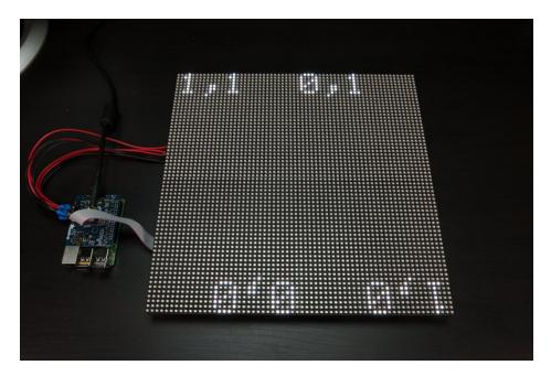
The text on a panel should be printed in its upper left corner. If the text is not in that corner then the rotation for that panel needs to be adjusted. You can see in the photo above the bottom row of panels do not have the right rotation. To fix this problem the matrix.cfg should be edited and a **rotation** of **180** degrees should be applied to those panels.
