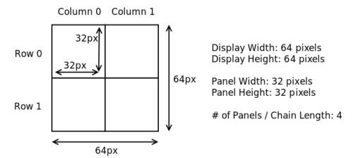
You can see four panels are combined to create a 64x64 pixel display. When the software runs it will take the Pi's video output and shrink it down to fit inside the 64x64 pixel display.
