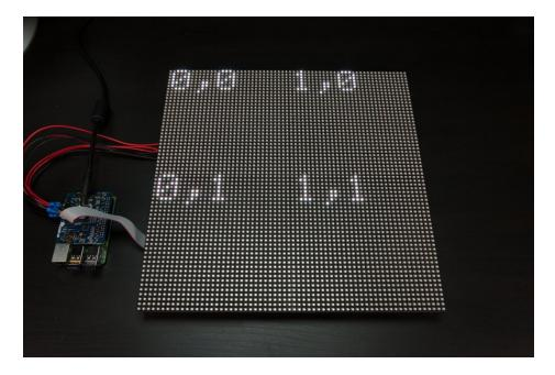
All of the panels have the correct orientation with text in the upper left. In addition the values on each panel are displaying the right order of columns and rows. Make adjustments to your matrix.cfg panel settings until the **displaytest** tool gives output just like the above.
