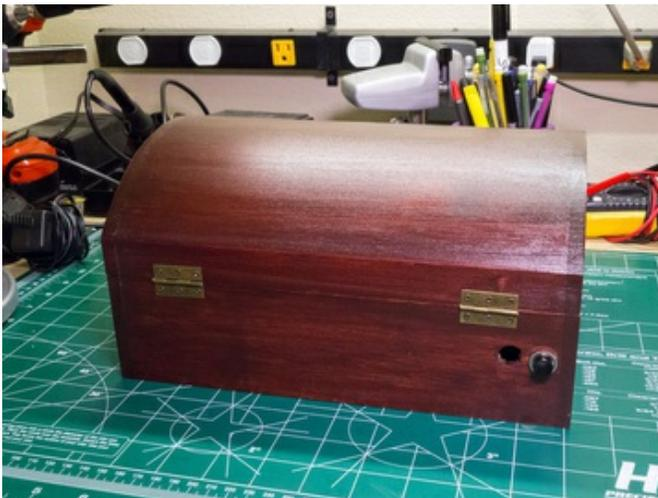
Drill a hole in the box to mount the push button. You can see I mounted mine on the back of the box where it can be reached while a user looks into the camera on the top.
