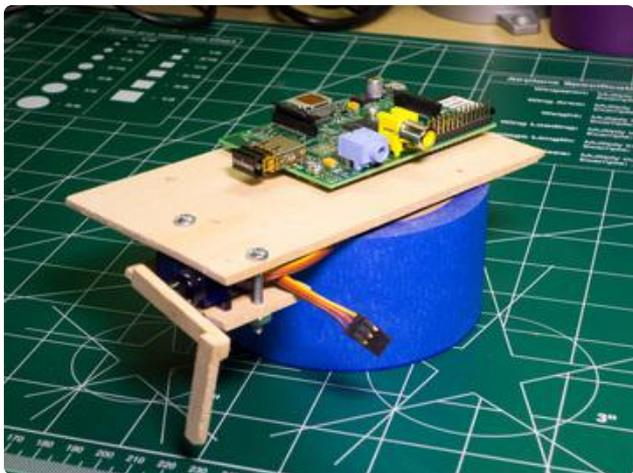
A few screws and a smaller board can act as a clamp to hold the servo in place.
