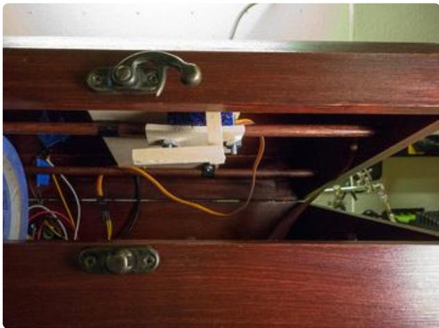
Latch in the locked position with a servo pulse width of 1100 microseconds.
