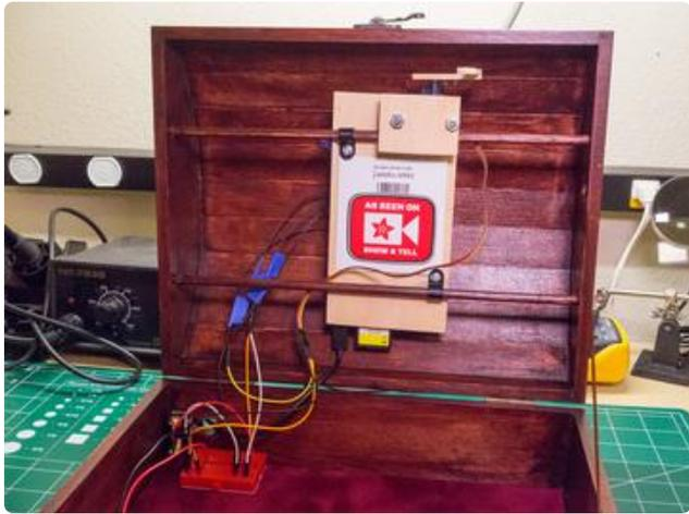
For the latching mechanism, mount a small dowel perpendicular to the side of the box. Attach a right angle of wood to a servo horn so it can act as a latch that swings down to catch the dowel, locking the box. See the pictures to the left to see the latch mechanism and dowel I built in my box.
