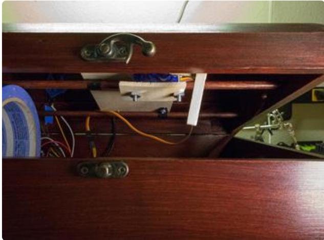
Latch in the unlocked position with a servo pulse width of 2000 microseconds.
