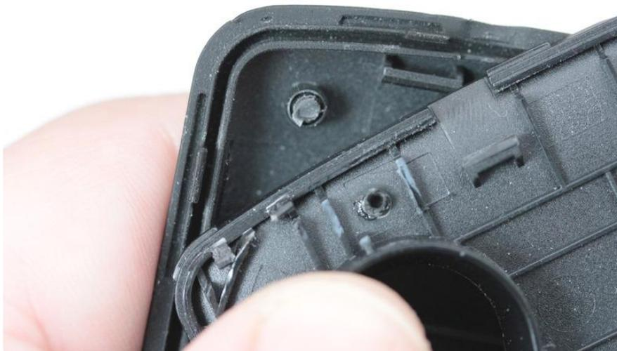
Being mindful of tolerances between parts is important. Manufacturers often set a high priority on making devices slim and smooth; this relief (below) was needed to make room for the battery.
