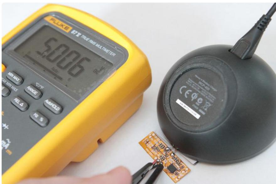
Cut a short length of red and black hook-up wire; connect the VCC and Ground from the charging receiver to the Micro USB pins we identified above.
