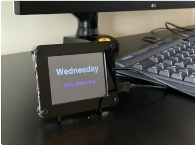
The code determines the local time by using the WiFi connection to query the Adafruit IO Time Service. It draws two labels to display the day of the week and the estimated time.
