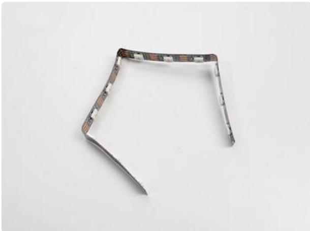
Cut the Neopixel strip down to 12 LEDs and remove the silicone casing. Using the middle piece as a reference, bend the Neopixel strip into a square so that each side sits nice and flush. It may take a few attempts, but the better it sits the better it'll look in the end.
