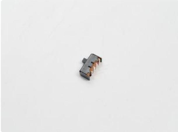
Bend the leads on the switch 90° so it'll fit on its ledge above the Trinket, and solder to the LiPoly backpack.
