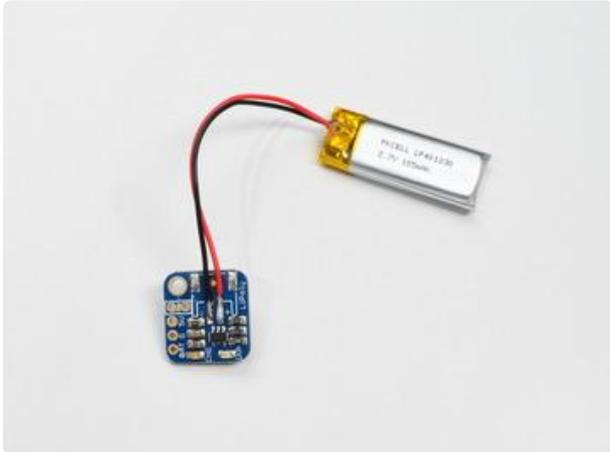
Also at this point, cut the trace between the two switch points so an on/off switch can be added :)
