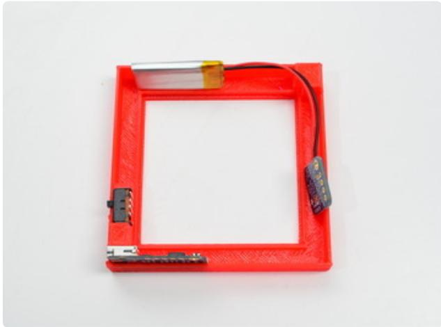
After cutting those traces, place the components back in the case as pictured and measure out the length of wire needed to get to the switch. The Trinket slides into the slots with a cut out to access the USB port.
