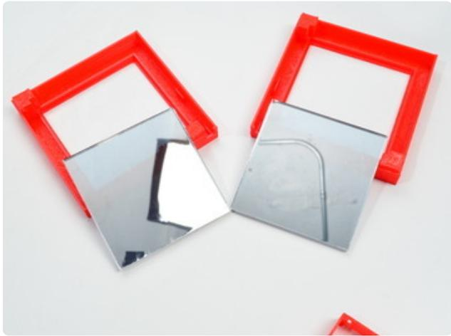
Place the mirrored acrylic into the case, and place each component in. The Trinket and switch have designated spots, whereas the Lipo battery and LiPoly backpack sit freely in the top and right (respectively) within the hollow frame. Clean the acrylic thoroughly to remove any dust/fingerprints. They'll be pretty obvious once it's lit up.
