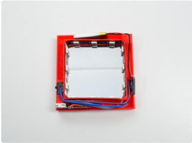
The two end pieces will house the electronics and mirrored acrylic, and the NeoPixel strips will be glued into the middle ring.
