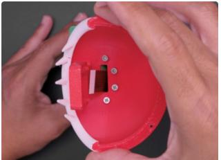
Fasten the mouth to the stem. The two screws on the outer side are M2.5x6mm long. The two center screws are M2.5x5mm long.
