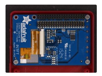
DO NOT insert screws all the way through standoffs! Reference the photo to see required depth.
