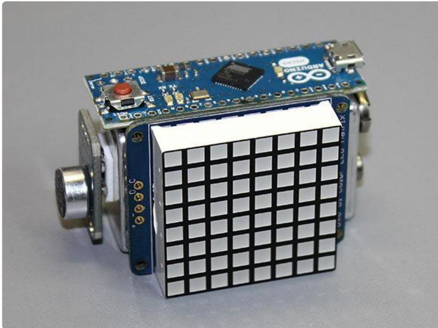
If you do attempt an extra-compact build like this, please keep in mind that the Arduino Micro includes a 5 Volt regulator, allowing it to be powered from a 9 Volt battery. Most small form-factor Arduino-compatible boards do not include a regulator, and will be damaged if you attempt to power them directly from 9 Volts! For such boards, either add your own regulator to the circuit, or use an appropriate battery pack: three alkaline AA or AAA cells in series, or four rechargeable NiMH cells.
