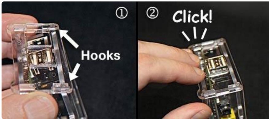
11. Install the opposite end of the case using the same technique. Top to bottom.
