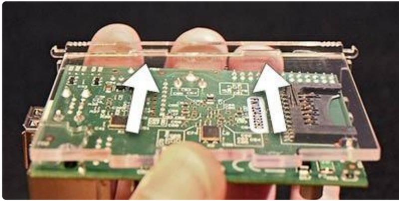
8. Turn the board over and install the top piece in a similar fashion. Or you can optionally leave the top off for full access to the GPIO and JTAG headers and the ribbon cable connectors.
