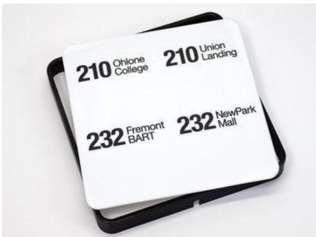
After cooling off and then soaking it underwater for a while, the paper peels away cleanly. The acrylic was slightly warped by all this heating, but was easily straightened out running under hot water.
