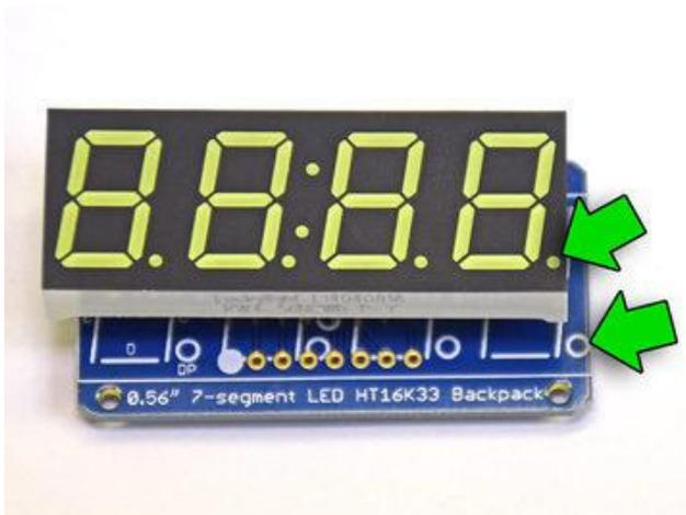
The 7-segment display/backpacks require some soldering. It is vitally important that the display be correctly oriented atop the backpack PCB! Use the decimal point markings (or the colons (:)) on the 1.2" displays) as an indicator. The IC chip should be visible on the back of the assembly, NOT covered by the display.
