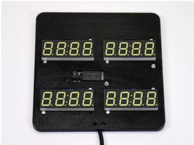
Keep track of the displays and their I2C addresses, since each is uniquely identified in the code. And remember when viewed from behind that the positions will be flipped left-to-right...the top-left display on the front of the clock will be on the top-right from behind.
