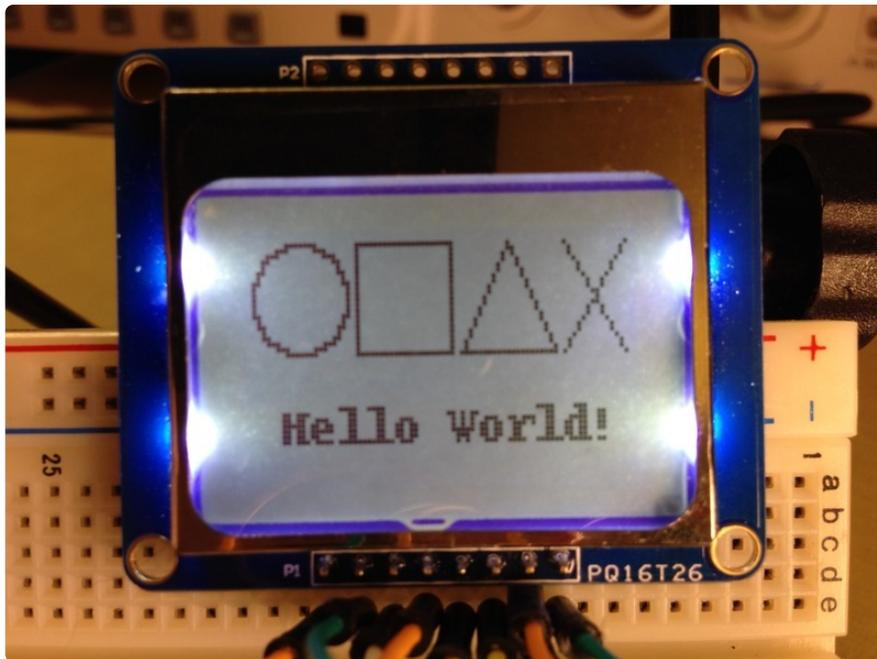
You should see your display draw a few shapes and a line of text like the image above shows. If you don't see anything, carefully check your connections to make sure the right pins are connected to the LCD. Also try adjusting the contrast value in the LCD's `begin()` call as it can sometimes be too low to be visible.
