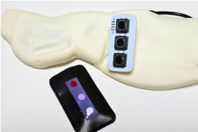
Sticking out of the molded foam piece is the button panel, which is just a PCB with three standard tactile switches inside a plastic and velcro sleeve.
