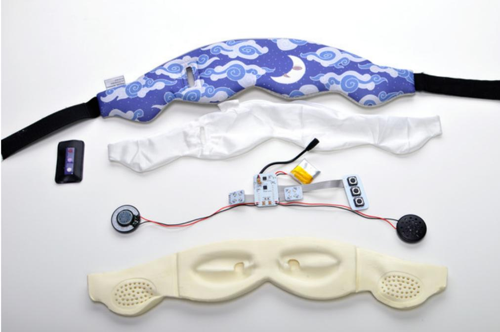
The device is comprised of four main sections: The outer dry-cleanable mask surface layer that comes in contact with your face and has velcro straps, the protective zippered mesh bag inside, the molded foam piece, and the electronic circuit inside. The parts came apart easily with hardly any tools-- we only used a pair of scissors once (to free the button sheath from the circuit board inside). We were able to put it back together just as easily, with no wonkiness or signs of having opened it.
