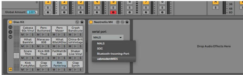
Click the **serial port** pulldown menu to see a list of **available serial devices**, and choose the **serial port** that corresponds to your **NeoTrellis M4**.
