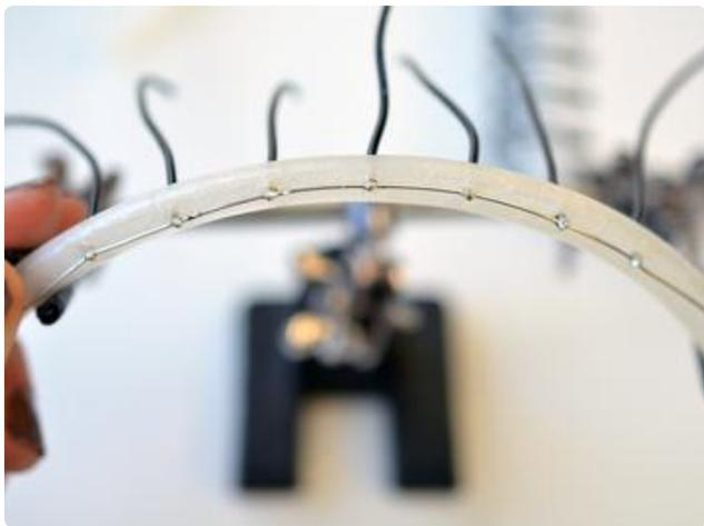
Be sure wire connections are tidy enough to nest snugly against the hair band, and solder connections in place.
