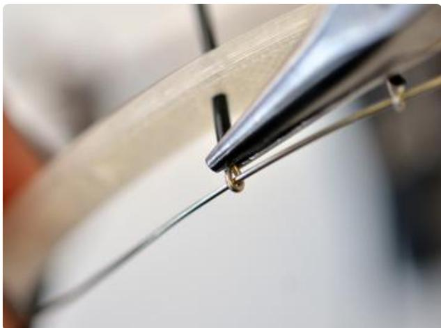
Strip the insulation from a long piece of solid-core hookup wire and clip it to one side of your headband. This will be the pixels' ground bus.
