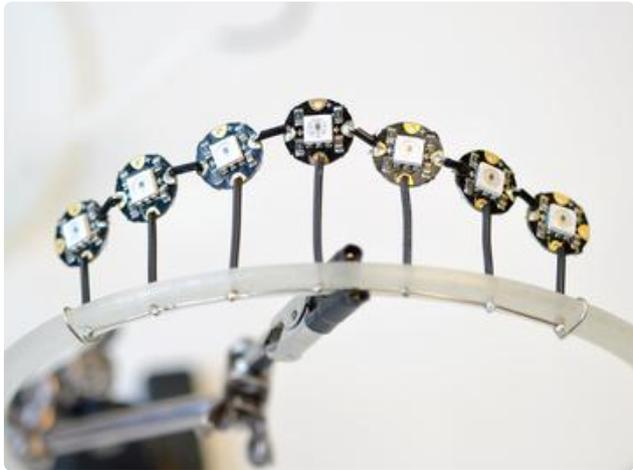
Next use bits of wire in the shape of staples to connect up the data lines.
