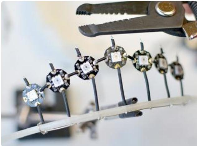
Solder wires from the + side of each pixel, and cut to length. Strip the ends and solder to one long power bus.
