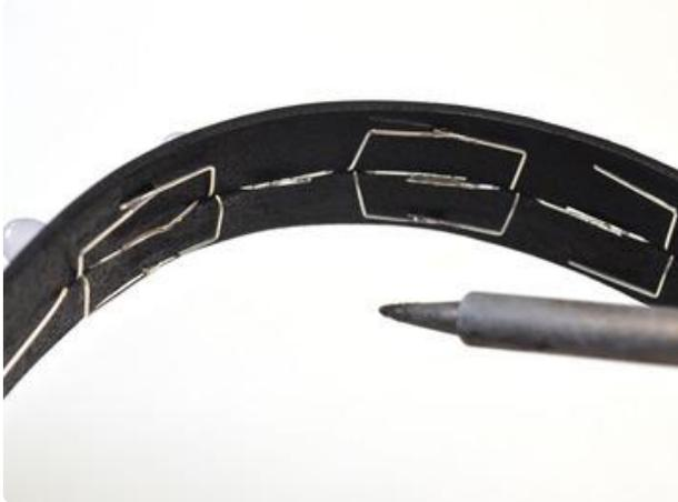
Solder overlapping wire leads while the collar is curved, using a pair of pliers to hold them close where necessary.
