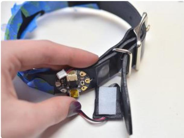
Wrap your battery in gaffer tape to protect it and provide strain relief to its wires.
