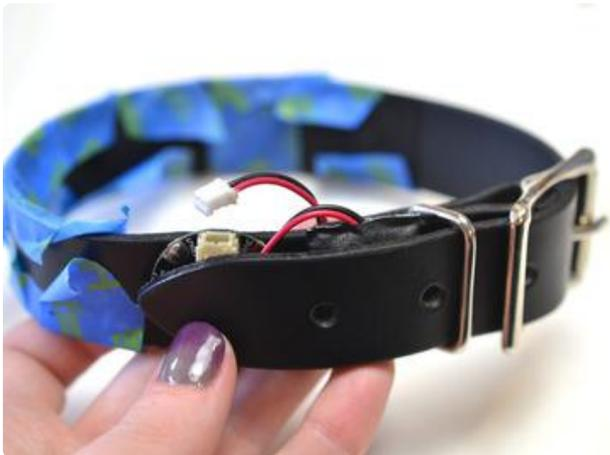
Use a piece of Velcro tape to affix the battery to the collar right next to the GEMMA. We arranged GEMMA and the battery so the collar slack covers/protects them. The battery wire wraps around the collar once, then plugs into GEMMA. This is how you turn the collar off/on.
