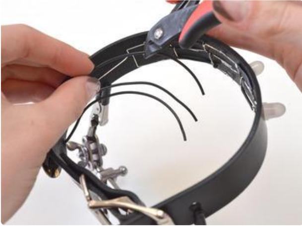
On the inside of the collar, trim and strip the other ends of the wire, then connect them up to the power bus, data in, and ground bus respectively (refer to circuit diagram). Wrap the wires around the pixel leads so they stay in place for soldering. Solder these connections and trim off any excess.
