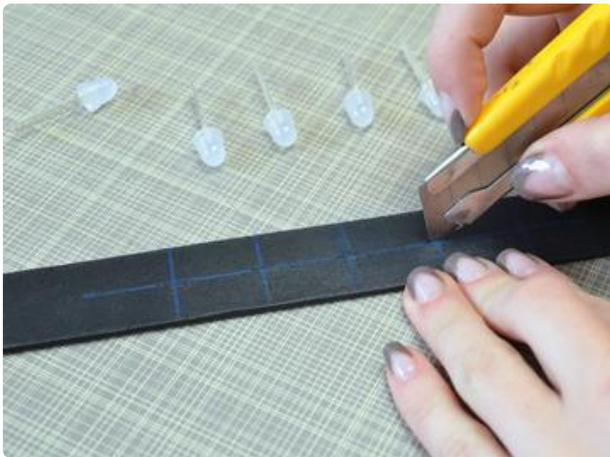
Use a utility knife to cut small horizontal slits in the collar at the marks. They should be just long enough for the legs of the NeoPixels to pass through, but not so long as they show on the front.
