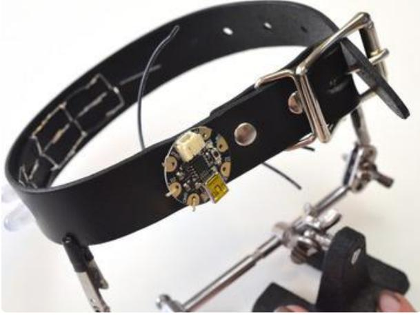
Pass the stripped ends of wire through GEMMA's pads marked Vout, D1, and GND, referring to the circuit diagram, and solder in place. Use flush snips to trim off excess wire.
