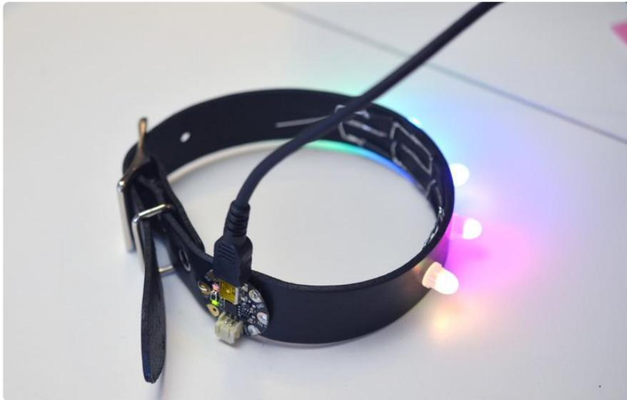
Plug your collar in with a USB cable and see if it's working! It should still have the program on it from testing earlier, and all five pixels should glow and animate. If they don't, use a multimeter to check your connections, and double check none of your pixels are in backwards!
