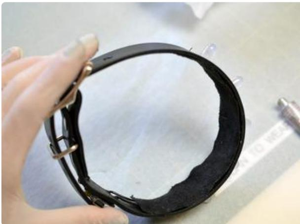
Once you know your circuit is solid, you can protect your delicate neck skin by gluing on a piece of fuzzy fabric (we used microsuede, a durable fuzzy microfiber) with E6000 craft adhesive. Painter's tape can come in handy for clamping over the edge. Allow to dry for 24 hours.
