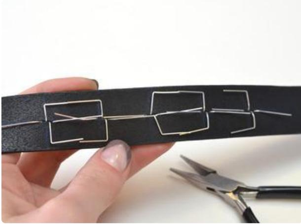
Bend the power and ground leads towards each other with a pair of pliers, and set the collar up, curved, in a set of helping hands. Trim the data leads to just overlap, but not get in the way of other legs.
