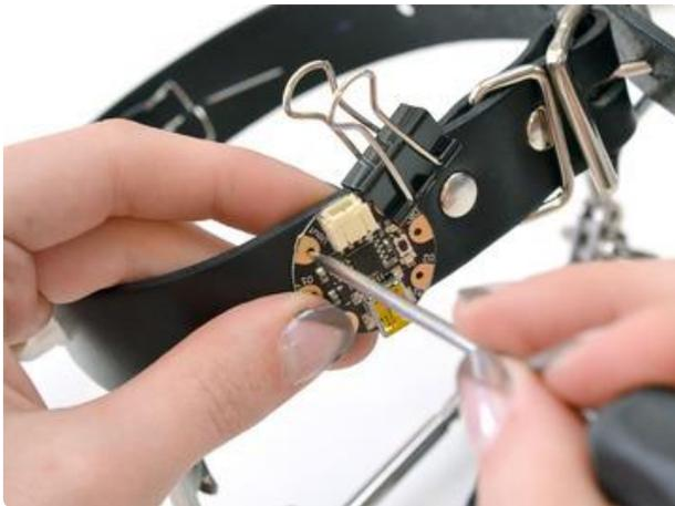
Use an awl to mark where wires will pass through the collar from GEMMA to the pixels.
