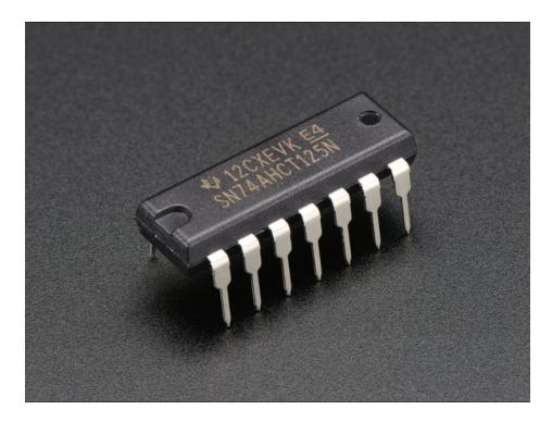
This is the 74AHCT125 (http://adafru.it/1787), a quad level shifter that can connect 3.3V and 5V devices of up to four channels.
