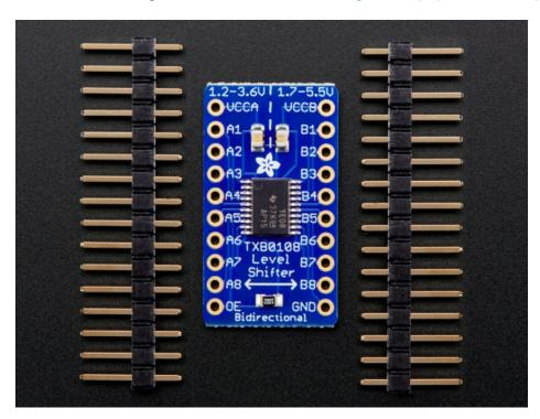
This chip can send messages in both directions, and works with pretty much any microcontroller and sensor pairing that need translation, however this guide just focuses on one possible pairing to NeoPixels.
