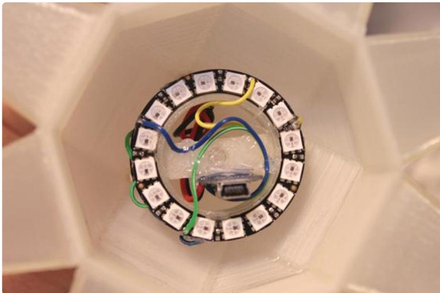
The LED rings will get a little warm... we need to let the star 'breathe' a bit. Either drill or melt vent holes in the top and bottom of the star.
