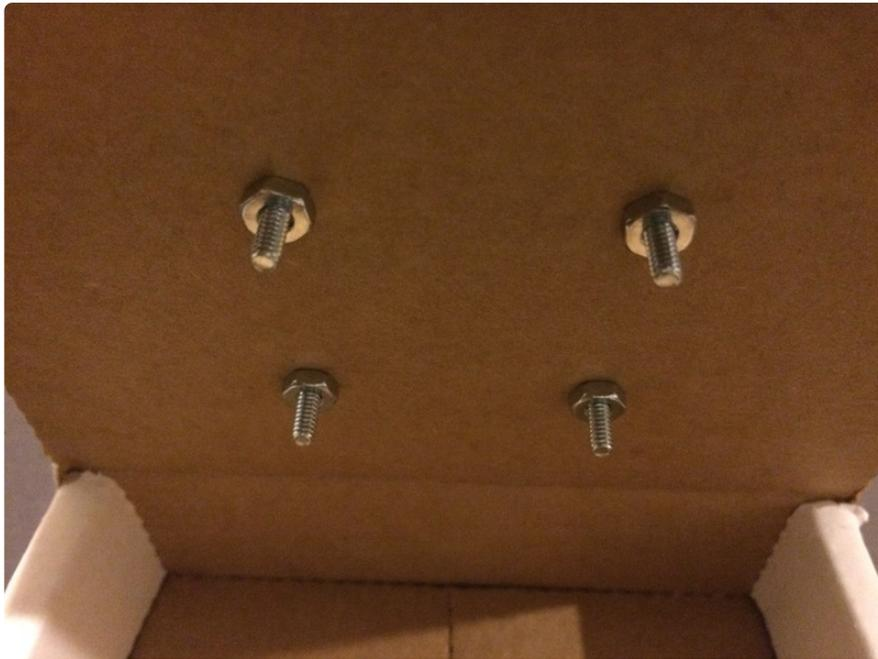
Note that the bolts can be mounted in a reverse orientation to easily allow external switches to be connected to the Circuit Playground via alligator clips.
