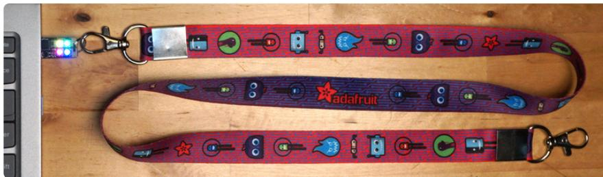
The Neo Trinkey works well as a base for a USB Kill Cord. It is small and unobtrusive. It can easily run the minimal code needed (which might also be none). It readily pops out of the USB port when pulled. And it has a convenient cut out for attaching a lanyard.
