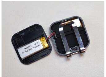
On the back of the clip, the black plastic is held securely in place by the metal clip. However it can be pried loose with the edge of a utility knife and delicately twisted away from the main body to reveal the 125mAh lipoly battery.
