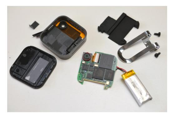
After removing the metal clip, the flexible gasket and circuit board can be delicately removed from the front plastic enclosure, inside of which lives the GPS antenna.
