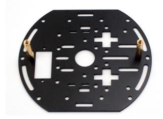
Attach two of the brass standoffs onto the black chassis layer.
