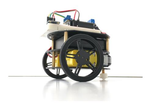
Get ready to race down the track with your **Feather** microcontroller-based **Mini Race Car!** You'll build this high performance racer, using the Bluetooth LE capable **Feather 32u4 Bluefruit LE** board, **Motor Driver FeatherWing**, and **TE HTU21D-F** temperature & humidity sensor to give you racetrack telemetry data.
