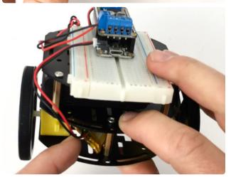
The AA batteries will supply power to the motors through the Motor Driver
