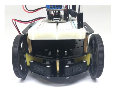
I used a couple M2.5 screws to secure the mounts to the robot (required a drill bit to clean up the holes in the 3D print). I wired up the left sensor to pin A4, and the right sensor to pin A5.
