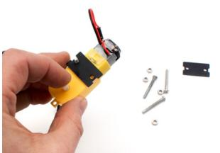
The metal panels go on the side with the red and black wires coming out.
