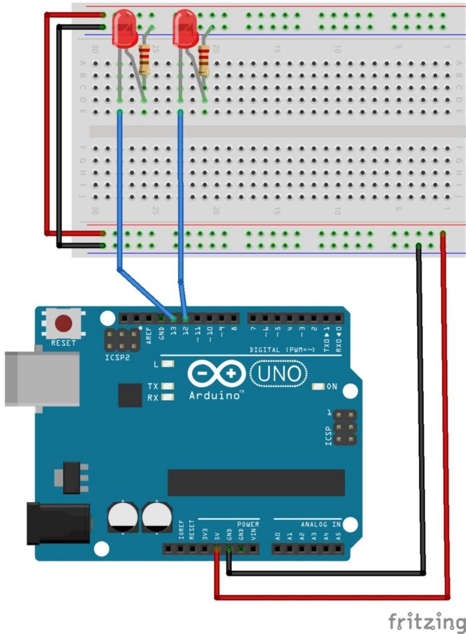
Then we'll create another state machine for a second LED that flashes at completely different rates. Using two separate state machines allows us to blink the two LEDs completely independent of one another. Something that would be surprisingly complicated to do using delays alone.
