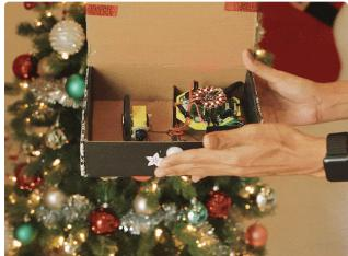
It uses a PIR motion sensor (http://adafru.it/189) to detect movement and a TT motor to spin a wheel. It also triggers lights and sounds making this an interactive gift box.
