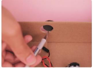
Measure a circle with 55.8mm (2.2in) radius and create a template to trace on to the side of the box as shown in the picture.
