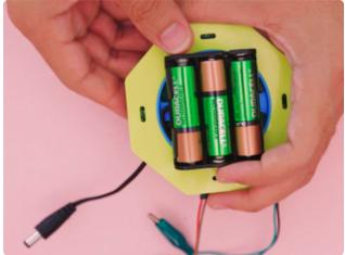
Thread the wires through the frame and use the included M3 screws to mount the 3xAA battery case to the bottom of the mount.
