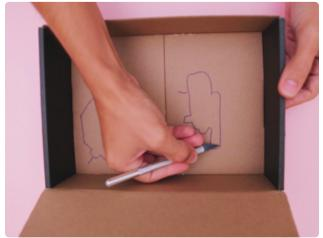
Start by tracing the Crickit board in the back corner of the box, with the power barrel arranged as shown in the picture.
