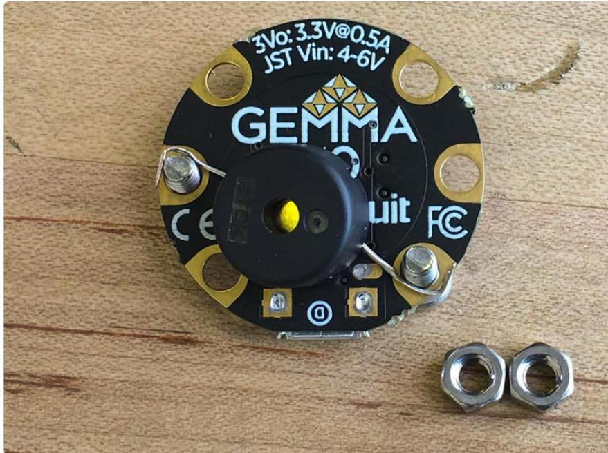
It doesn't matter which leg of the buzzer goes to which pad, it is not polarized.
