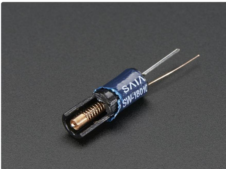
By connecting one leg to analog pin A0 and the other to GND, we can code the Gemma M0 so that it monitors the analog value of the A0 input pin — when the spring vibrates it will send the analog pin to ground, and so the analog voltage value will decrease. When the value goes below a certain threshold, the code will send a pulse width modulated (PWM) tone signal to the piezo buzzer on D0 to make it sound the alarm.
