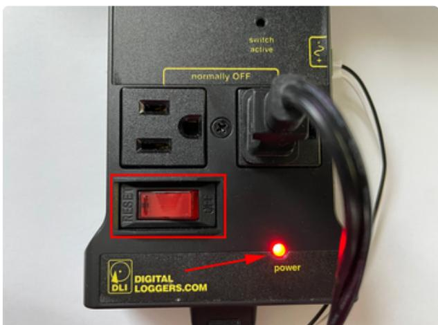
Make sure the Power Switch is in the On position for both the outlet and the appliance. The Power LED should be lit.
