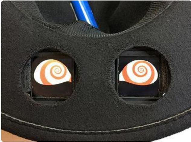
Make sure the screens align with the holes before the glue sets. If I were doing this over, you'd see a stencil around the screens blocking stray light. This was my prototype and I'd painted over things instead.
