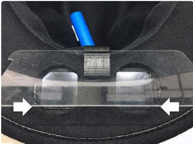
Once the board was securely in place, I used the same 3D-printed doodad...but only for holding the screen glass, not the circuit board. Make sure the clip is straight before the glue sets.
