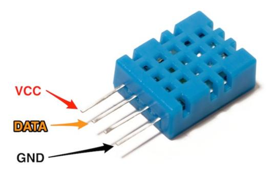
Connect the VCC pin to the Raspberry Pi 3.3V pin, GND to GND, and DATA to pin number 4 on the GPIO connector. Finally, connect the 4.7K Ohm resistor between the VCC and DATA pins. The picture below shows the final result for the sensor:
