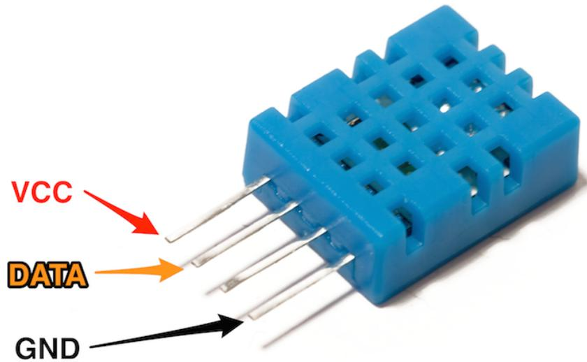
Connect the VCC pin to the Raspberry Pi 3.3V pin, GND to GND, and DATA to pin number 4 on the GPIO connector. Finally, connect the 4.7K Ohm resistor between the VCC and DATA pins. The picture below shows the final result for the sensor:
