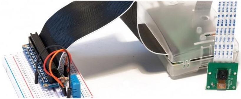
There are lots of devices on the market that allow you to monitor your home from a central interface. In this article, we are going to make our own DIY version of such devices. To do so, we will use the latest Raspberry Pi board, the B+ model, and the official [Raspberry Pi camera module](#) (). We will also perform some measurements from a temperature and humidity sensor.
