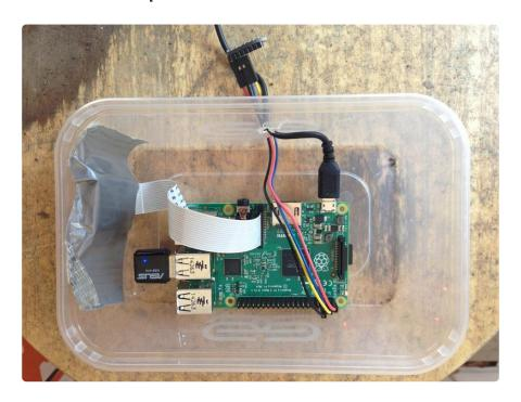
I've just used an old plastic food carton and cut holes in the side and front for the cabling and camera. As this box is outside I've kept the number of holes to a minimum. It's worth having long enough jumper cables so the temperature sensor can hang outside the box. I was getting slightly high readings when I had it in the box with the lid on due to the small amount of heat produced by the Pi.
