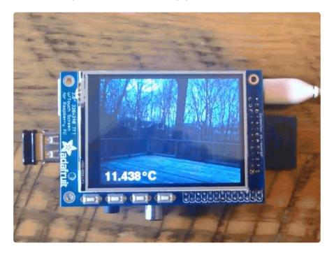
This project uses two Raspberry PIs - a sender and a receiver. The sender has a Raspberry Pi Camera and an MCP9808 temperature sensor to publish data to adafruit.io. The receiver, a dashboard somewhere else in the world, subscribes to this data feed and displays it.
