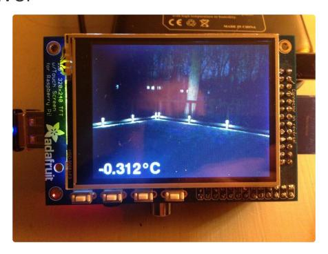
As you can see from the picture, the receiver will be taking the images and temperature readings from the feed and displaying them on the PiTFT via Pygame. The overview from my Raspberry Pi Pygame UI Basics () tutorial will get your environment all set up and running sweetly.
