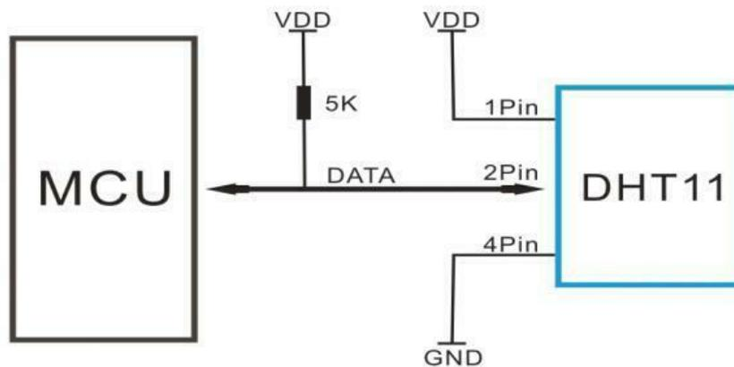
In the diagram above, "MCU" is the microcontroller, i.e your Arduino UNO, Feather M4 Express, Raspberry Pi, or whatever you are connecting the DHT11/22 sensors to. **There's only one pin used for data.** This is a digital pin, so is either HIGH or LOW. The sensor readings (humidity, temperature) need to be sent over as a stream of 1's and 0's. But how is that done? Sure, HIGH=1 and LOW=0, but how does the MCU know **when** to read the DATA line? The answer is timing.
