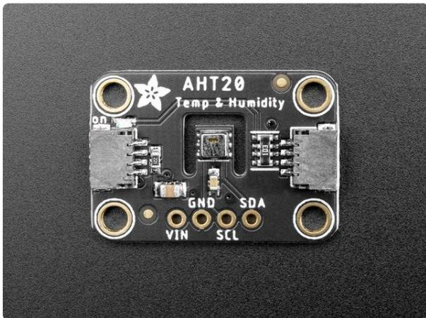
[Adafruit AHT20 - Temperature & Humidity Sensor Breakout Board](#)
