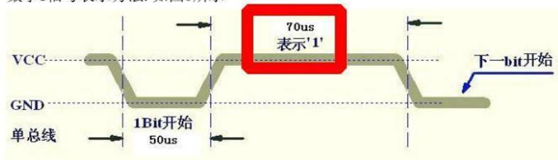
So a 0 is represented by a HIGH time of 26us-28us and a 1 is represented by a HIGH time of 70us. That "us" is units of **microseconds**. To put that in some perspective, Arduino's much used `delay()` (<https://adafru.it/COV>) function uses units of **milliseconds**. The smallest delay you can program with that function is:
