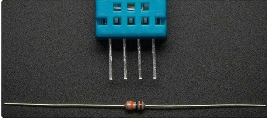
Even though these sensors typically have 4 pins, only 3 are used. For example, here is the wiring diagram from the [DHT11 datasheet \(https://adafru.it/aJY\)](https://adafru.it/aJY):
