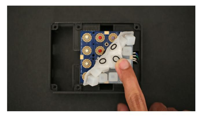
Install Elastomers to Trellis PCB
