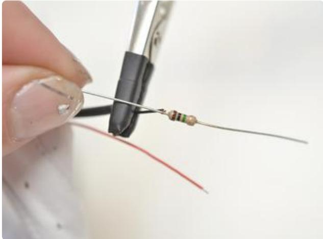
Wrap the wire end around one of the resistor's leads (doesn't matter which one), and situate the two in the grasp of your third hand tool.
