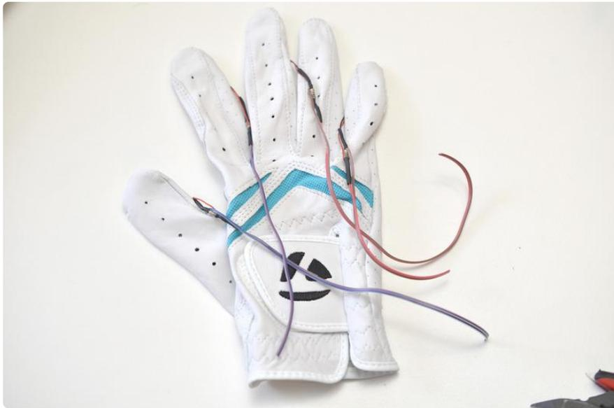
Put the glove on and finesse the wires into a position that reduces strain and lets your hand move. Use painter's tape or masking tape to hold the wires in place as you route the ends towards the analog inputs on FLORA.
