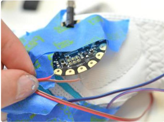
Solder each piezo's red wire (or whatever color your red wire became when you extended it) to a different analog input according to the circuit diagram.
