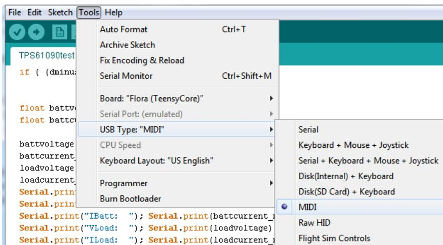
Load the code below into your Arduino IDE. Before uploading the code to the board, press the mini reset button on the Flora to launch the bootloader again. There's a 10 second window to then click Upload. If you miss it on the first try, just try again!
