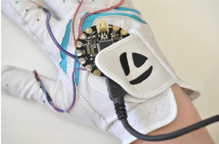
Your USB cable will be plugged in while you use the drum glove. You may want to grab a USB extension cable for more freedom of movement! For a similar, yet wireless, project, try the [3D Printed Wireless MIDI Controller Guitar](#) ().
