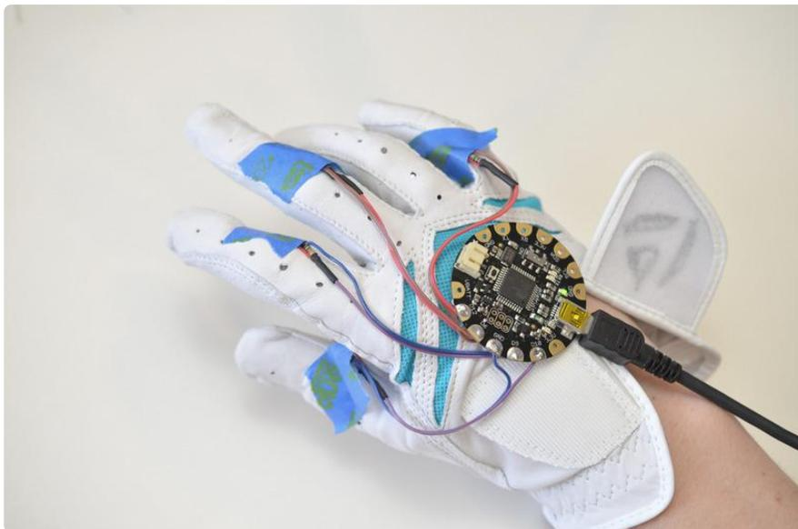
Before sewing FLORA to the glove, plug in via USB and test your rig using the code on the next page. You'd hate to have to unstitch anything if anything needs re-soldering!
