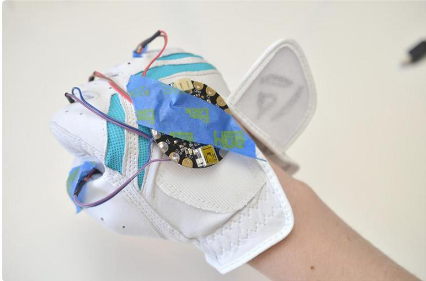
Once your glove is functioning properly, it's time to tack everything down. Put the glove on and position FLORA so that the wires don't tug when you make a fist. Tape it down so it stays put before stitching.
