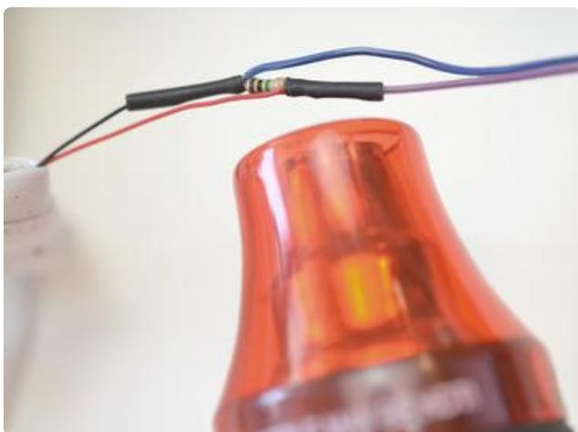
Now it's time for the other wire-- wrap the piezo's red wire and the other wire around the other side of the resistor, remembering to add a piece of heat shrink tubing before soldering.
