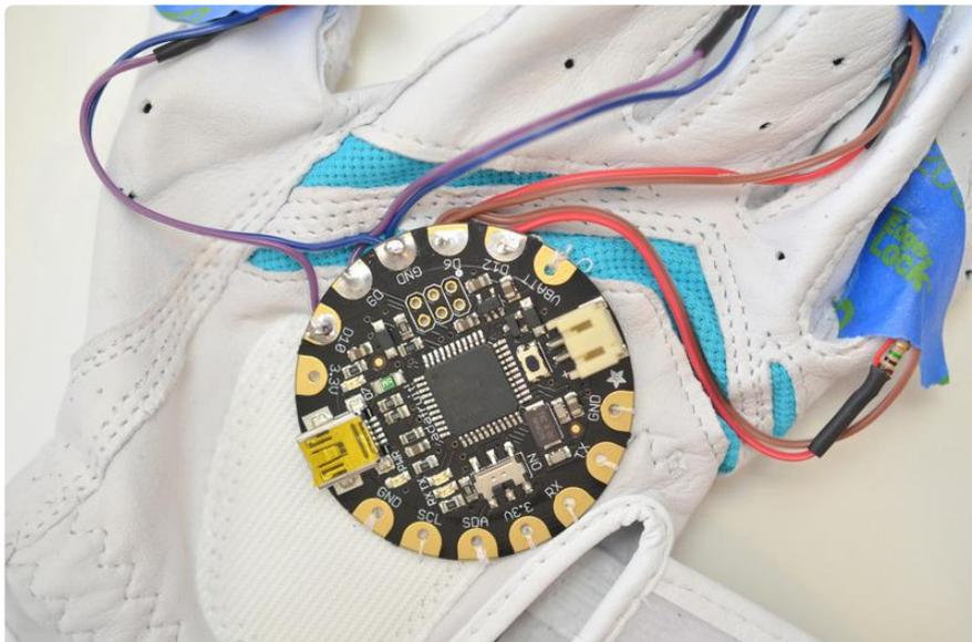
Use plain thread to stitch FLORA's unused pads to the glove. On the side where all the wires come in, stitch around the wires instead of through the pads.
