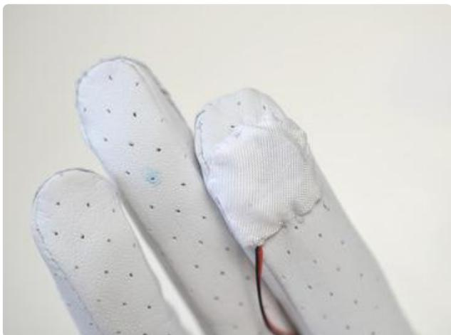
Stick the piezo in the pocket, then finish stitching it shut, leaving the wire sticking out towards the back of the hand. Tie off and cut your thread.
