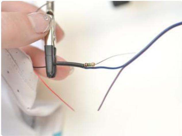
Once soldered, clip the resistor lead short and shield the junction with the heat shrink tubing you added earlier.
