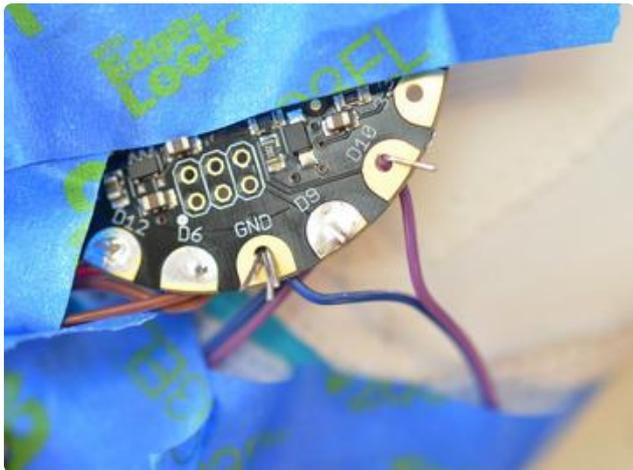
Solder all the piezo's black wires to ground.
