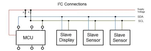
Inter-Integrated Circuit ( $l^2C$ ) is yet another serial communication capability, and is often called Two Wire Interface (TWI). It's synchronous like SPI; the main device generates and provides a clock. If you've worked with it you'll have noticed the clock (SCL) and data (SDA) lines. That's where the *two-wire* in the name comes from. Because there is only a single data line,  $l^2C$  is half duplex, meaning that data can only go in one direction at a time.
