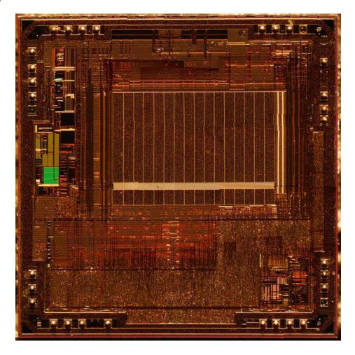
Above is a picture of the ATmega328 silicon die/chip. This is what's inside that large, long IC on many Arduino UNO compatibles and the small square IC on an Adafruit Metro Classic (https://adafru.it/METROXMETR) (below) and on an Arduino pro mini. Both packages appear on a number of other comparable microcontroller boards.
