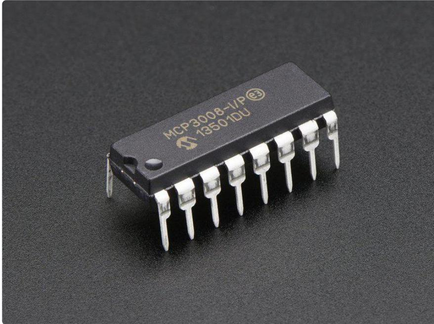
Need to add analog inputs? This chip will add 8 channels of 10-bit analog input to your microcontroller or microcomputer project. It's super easy to use, and uses SPI so only 4 pins are required.
