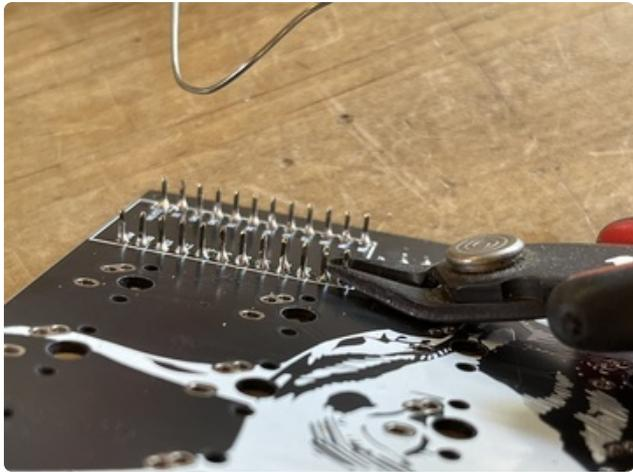
After that, flip the board over and solder the headers to the PCB. You can cut off the excess leg length if you'd like to, but doing so isn't necessary.
