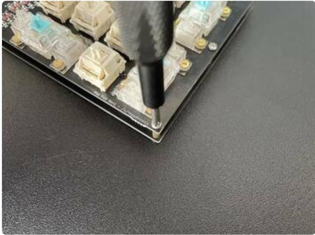
Finally, attach the two halves of the case with the standoffs and screws included in the kit and put the keycaps on.
