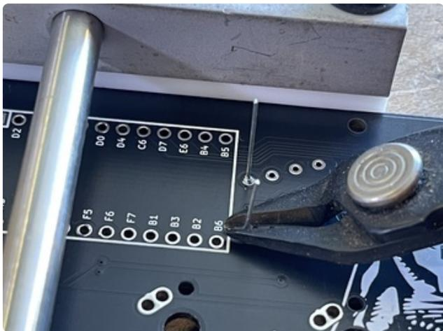
Next, solder in all the diodes. Make sure the black band is on the side of the square soldering pad. After soldering all the diodes, go over to the other side and cut off the excess legs.
