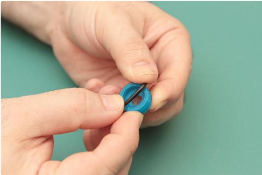
Trim the servo horn down a bit so that it will fit inside the hub.
