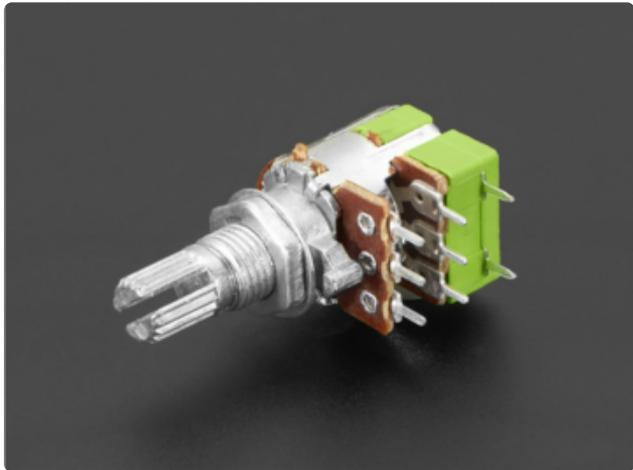
Some applications, such as audio, benefit from adjusting two potentiometers via one shaft. Those are called **dual potentiometers**. More rarely there could be three or more stacked on one shaft. These come in linear and logarithmic tapers.
