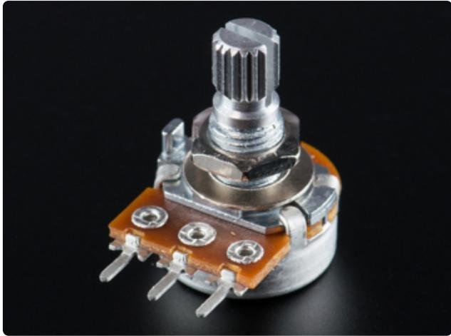
Exactly like normal, fixed resistors, potentiometers are rated for a maximum resistance measured in Ohms. Often it is in thousands of Ohms (1000 = 1K), or millions of Ohms (1,000,000 = 1000K = 1M megohm).
