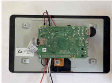
Gently turn the Pi upsidedown and screw it to the mounting holes on the back of the touch screen. This is not the way it's designed to be mounted, so you'll need to carefully manage the wires. I could only get three screws to bite, but that should be plenty for this project.
