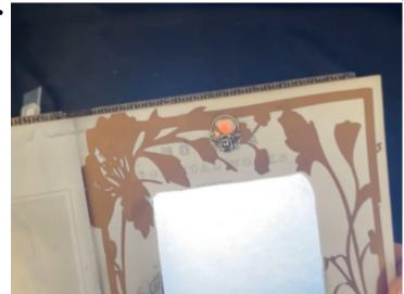
To highlight the NeoPixel indicator light, I used a small ring from my scrapbooking drawer filled with UV resin. The resin cures in minutes when you shine a blacklight on it and does a great job of pulling the light up into a dome so it diffuses and refracts in a magical way.
