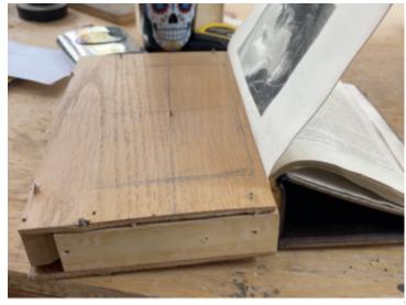
To stabilize the pages, I built a box out of some wood scraps and screwed it all together around the pages I wanted to cut. I put a screw right through the center as well -- we're cutting that part out so it's okay to put a hole in it.
