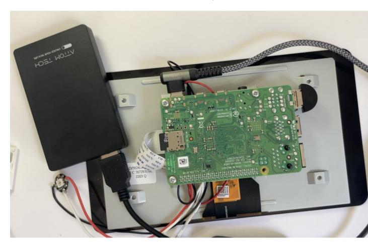
Plug your USB cable into the Pi's power port and plug the other end into your on/off switch. Then plug another cable from the switch to the battery's "out".
