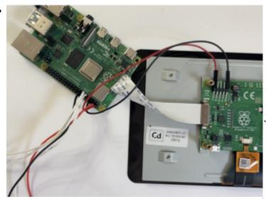
Plug the other end of the cable into your touch screen as shown. Plug the jumper cables into 5v (red) and G (black).
