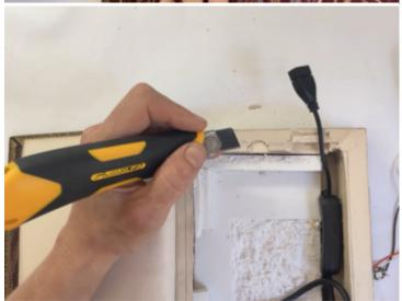
I used my dremel to hollow out a divot in the cover for my rare earth magnet, and glued it securely in place with E6000. Then I carved out a hollow for my NeoPixel and a hollow for the reed switch, which I made sure to line up with the magnet. The magnet will activate the switch when the book is closed and cause the project to sleep.
