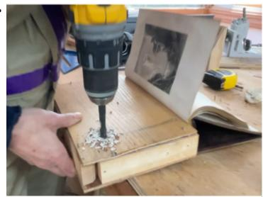
Next I drilled a hole right in the corner so I could get my jig saw blade through. The corners are the hardest part with the saw, and I wanted them rounded, so using the drill made this easier. I could just cut straight from hole to hole and the drill holes made the corners rounded for me.
