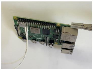
Here's a great pinout diagram for the Raspberry Pi 4. (https://adafru.it/18Dk) Solder your switch wires to G and GPIO 17: the 5th and 6th pin on the inside row of pins.
