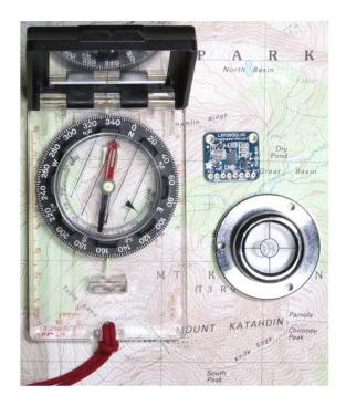
The <u>LSM303</u> (http://adafru.it/4413) breakout board combines a magnetometer/ compass module with a triple-axis accelerometer to make a compact navigation subsystem. The I2C interface is compatible with both 3.3v and 5v processors and the two pins can be shared by other I2C devices. Combined with a 3-axis gyro such as the <u>L3GD20</u> (http://adafru.it/1032), you have all the sensors you need for a complete IMU (Inertial Measurement Unit) for use in aerial, terrestrial or marine navigation.
