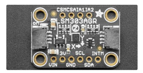
In addition to being a physically smaller and easier to lose chip, there are a few other difference as well. The chip itself exposes an interrupt pin for the magnetometer (INTM) (perhaps a feature of the new magnetometer sensor inside?) as well as chip select pins for both the accelerometer and magnetometer (CSA and CSM respectively).
