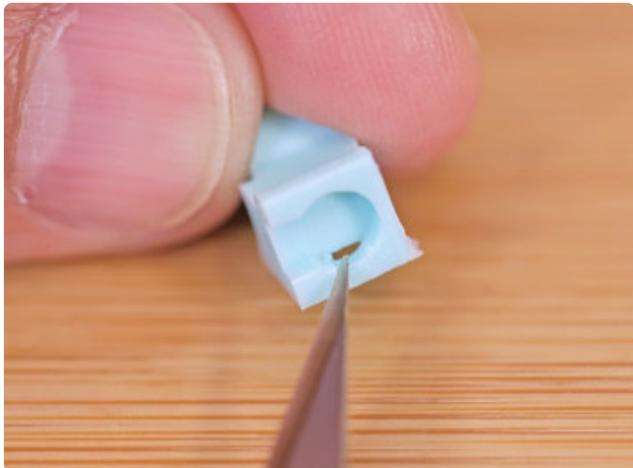
To remove supports around the face and arms, use Precision Flat Pliers to grip and pull away from the parts.
