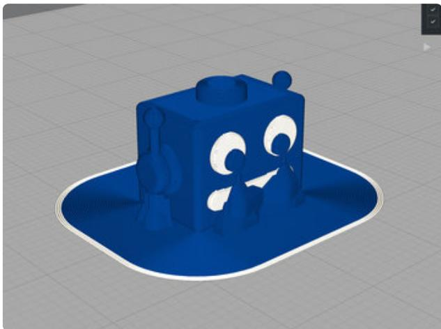
Rotate the head so it sits upright. Make sure to have the supports set to **Touch bed plate**, otherwise the head cavity will generate too much support material.
