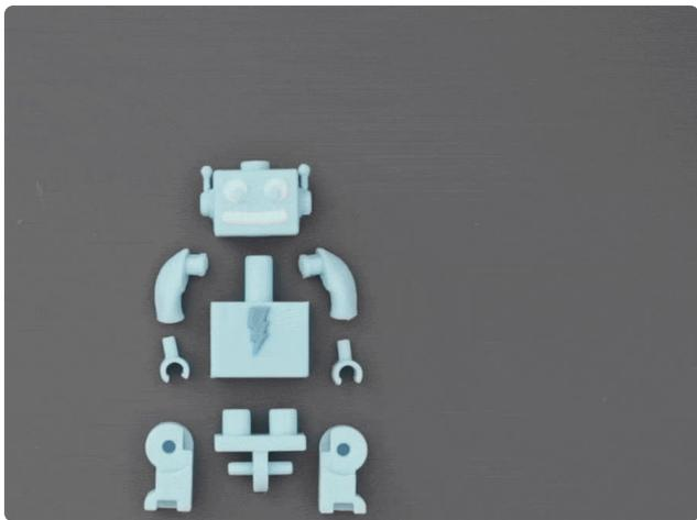
First attach the hands to each arm. If the tolerances are a bit too tight, we recommend removing a tiny amount of material from the wrist section on the hand. Remove a little at a time until it has a tight fit inside the arm.
