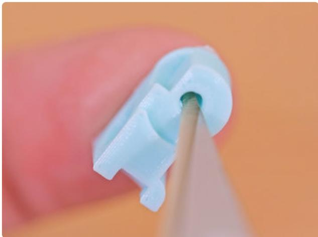
If the tolerances for the legs seem too tight, check the inside of the connector for where the z seam might be. Use the tip of the hobby knife clean around the hole.
