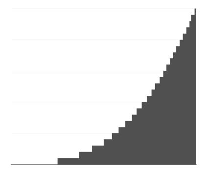
"Luxury" LED drivers such as the PCA9685 (https://adafru.it/dUG) and TLC5947 (http://adafru.it/1429) use 12-bit PWM (4096 output levels) to minimize the effects of quantization. More advanced drivers like FadeCandy use dithering to 'fake' a wider dynamic range
