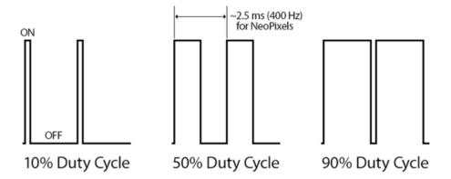
When you program in a "halfway" level (like 127 out of the maximum 255), you are indeed getting something very close to a proper 50% duty cycle. The LEDs are doing the correct thing.
