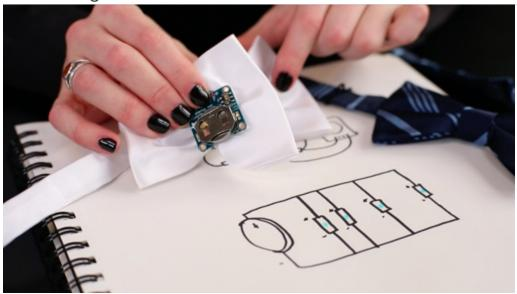
Two or four LED sequins are wired in parellel with the coincell battery. Stitch postitive traces to SW and negative traces to Gnd on the coincell breakout. Practically, inside the bow tie, the stitched threads will form a shape something like this:
