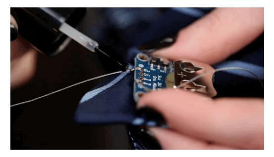
Seal your knots with clear nail polish, being careful not to get any on the pads of the circuit board. LESS IS MORE.
