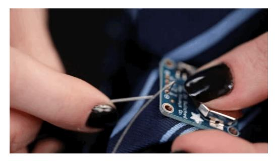
Double check your needle fits through the holes on the battery board—they are on the smaller size. Thread your needle with conductive thread and connect it up to either the SW or Gnd pad on the board and get to stitching towards your sequins according to the circuit diagram and your desired layout.
