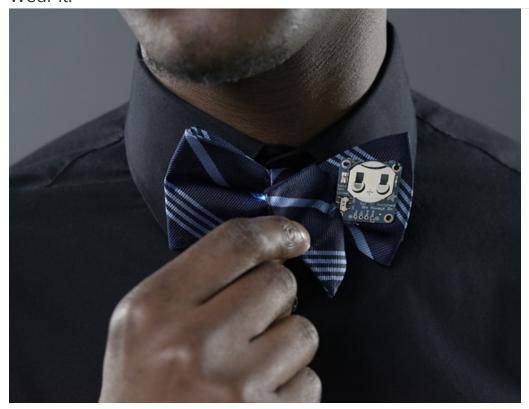
Once all your thread tails are cut, you can insert the coincell battery into its holder and flip the small power switch. Your sequins should light up! If they don't, switch it off and check your circuit for shorts and loose stitching and try again.
